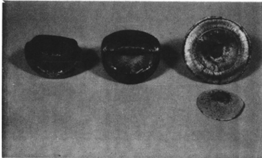
1.50 in. diam. pipe 1.25% NQ left, 2.5% NQ middle, 5% NQ right
